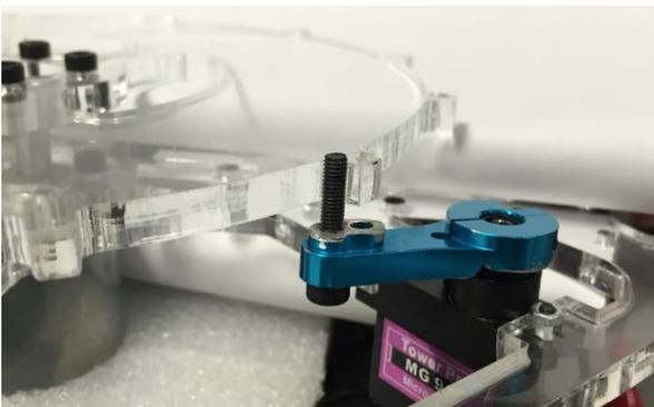
Fig.5 Braking mechanism acting on tooth barrier
