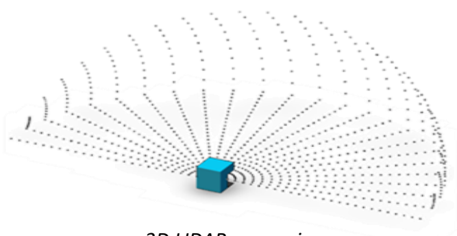
3D LIDAR scan using external rotary actuator
