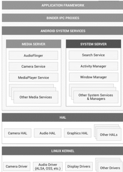
Fig. 3 Mobile Operating System Core Structure
