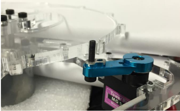
Fig.7 Braking mechanism acting on tooth barrier
